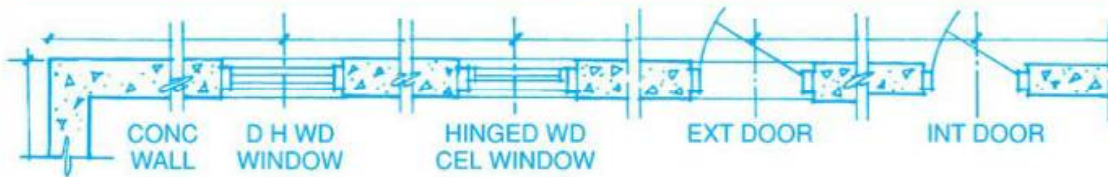
DOORS AND WINDOWS IN CONCRETE WALL
