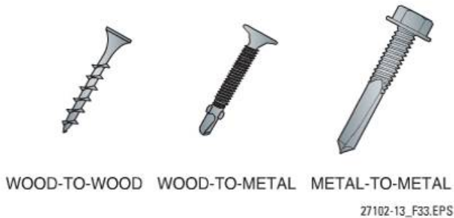
Figure 33 Typical deck screws.
